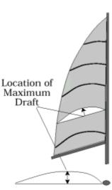
• TRIM: Controlled by the mainsheet and the traveler. Although closely interrelated, each control has a distinct effect on the mainsail's characteristics. It is instructive and fun to work the controls and observe the effects
