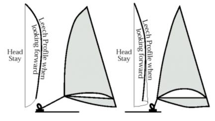
Jib lead aft flattens the foot and loosens the leech because the sheet pulls aft more than it does down. Jib lead forward loosens foot & tightens the leech because the sheet pulls down more than it does aft.
